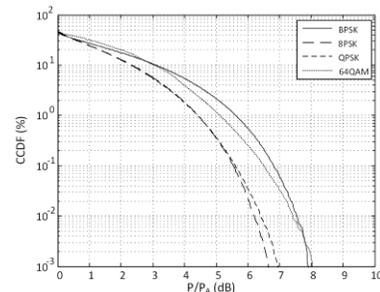
Fig. 2. Measured CCDF of modulated signals with  $\beta = 0$  and 500 KBPS symbol rate.
