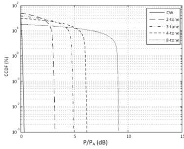
Fig. 3. Measured CCDF and PAPR of multi-tone signals.
