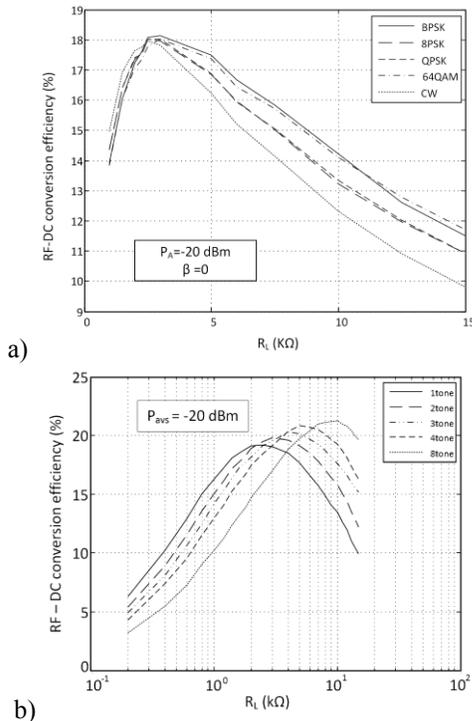
Fig. 4. Measured RF-DC conversion efficiency of a) randomly digital modulated signals and b) multitone signals.
