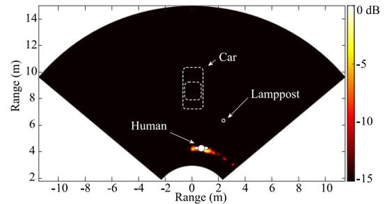
Fig. 5. Human target extracted with standard deviation of 10 sequencing scans.
