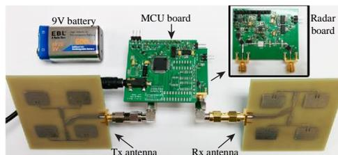
Fig. 1. Photo of the 5.8-GHz multi-mode radar prototype.
