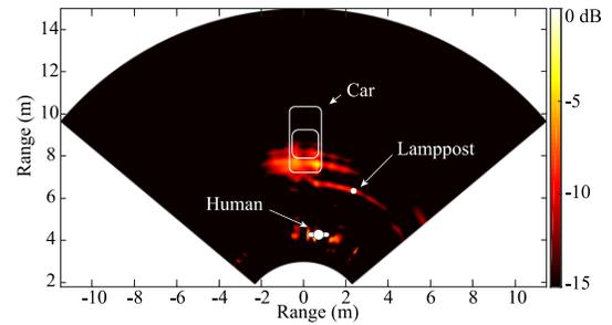
Fig. 4. Measured result of the short-range localization experiment with a human subject and two object targets using the proposed radar prototype.
