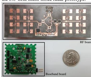
Fig. 2. Photo of the 24-GHz multi-mode radar prototype.
