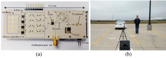
Fig. 3. (a) Photo of the proposed radar prototype. (b) Experimental environment of short-range localization with a human subject and two object targets using the proposed radar prototype.
