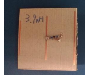
Fig. 3. Prototype of the fabricated 2.45 GHz rectenna.
