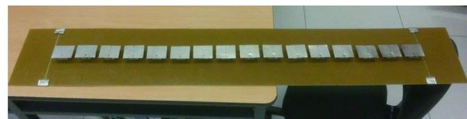
Fig. 4. Implemented high gain 16-element patch antenna array.
