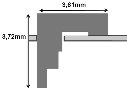
Fig. 2. MWT first solution, side view.
