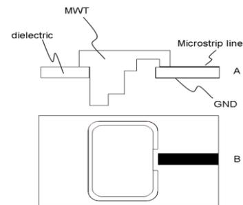
**Fig. 1. A, side view of the MWT; B, PCB with waveguide opening.**
