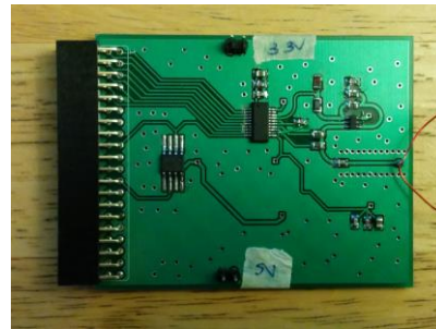
Fig. 3. PNS receiver printed circuit board with limited analog frontend circuitry
