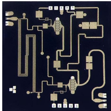
Fig. 2. Photo of the GaN MMIC Doherty PA designed according to the technique proposed in [3,4]. Measurements results showed that  $PAE_{avg} > 32\%$  was obtained across the 5.8-8.8 GHz frequency range when employing a 20 MHz 8.54 dB PAPR signal. The chip dimensions are 2.9 x 2.9 mm.
