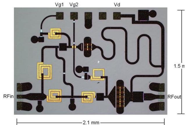
Fig. 1. Photo of the GaN MMIC Doherty PA in [6]. Measurements results showed that  $PAE_{avg} > 35\%$  was obtained across the 6.8-8.5 GHz frequency range when employing a 10 MHz 7.8 dB PAPR signal. The chip dimensions are 2.1 x 1.5 mm.
