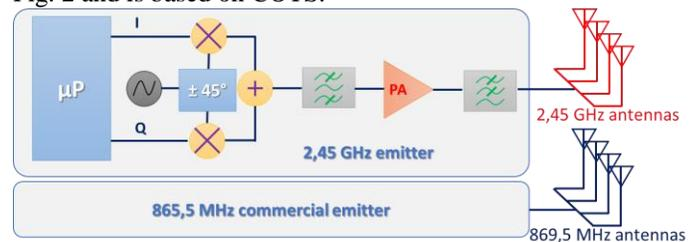
Fig. 2. Dual-band transmitter with 2.45 GHz emitter detailed architecture.
