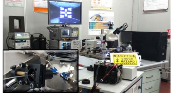
Fig. 1. Photo of experimental set-up for measuring DC characteristics, S-parameters and extrapolation of N-parameters; particular of the optical focusing system on the down-left corner.
