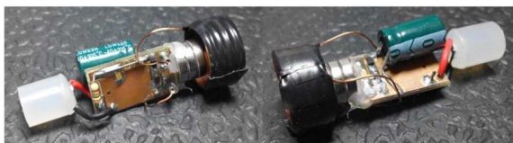
Fig. 3. Levitated object. It contains the receiver coil (covered with black tape), the resonant circuit, the permanent magnet (three neodymium disks), a LED with a silicon diffuser and a rectifier circuit to power the led. Total weight is 80 gr.
